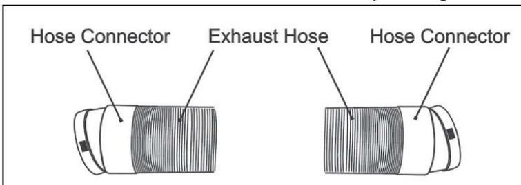
3. Align the slots on the hose connector to the tabs on the air exhaust and snap the hose to the unit.
